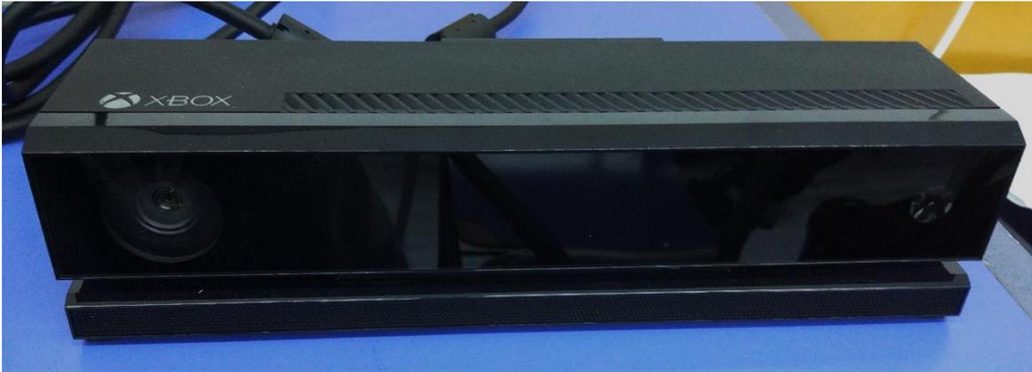
**Figura 3:** sensor Kinect v2 (Xbox). Microsoft Corporation, USA.
